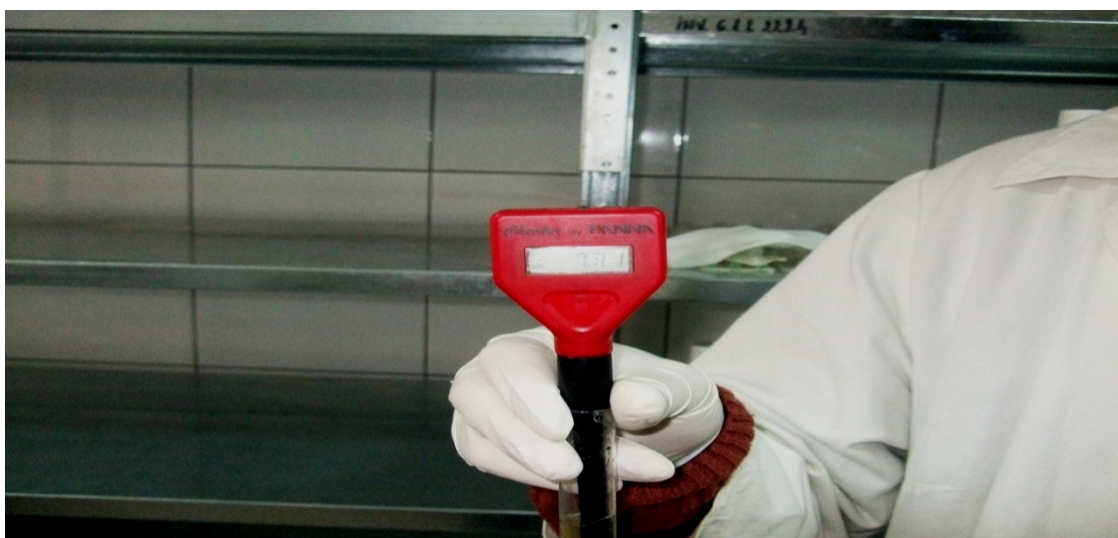
Photo 1. Checker-type pH-meter, Hanna production, with electronic display
